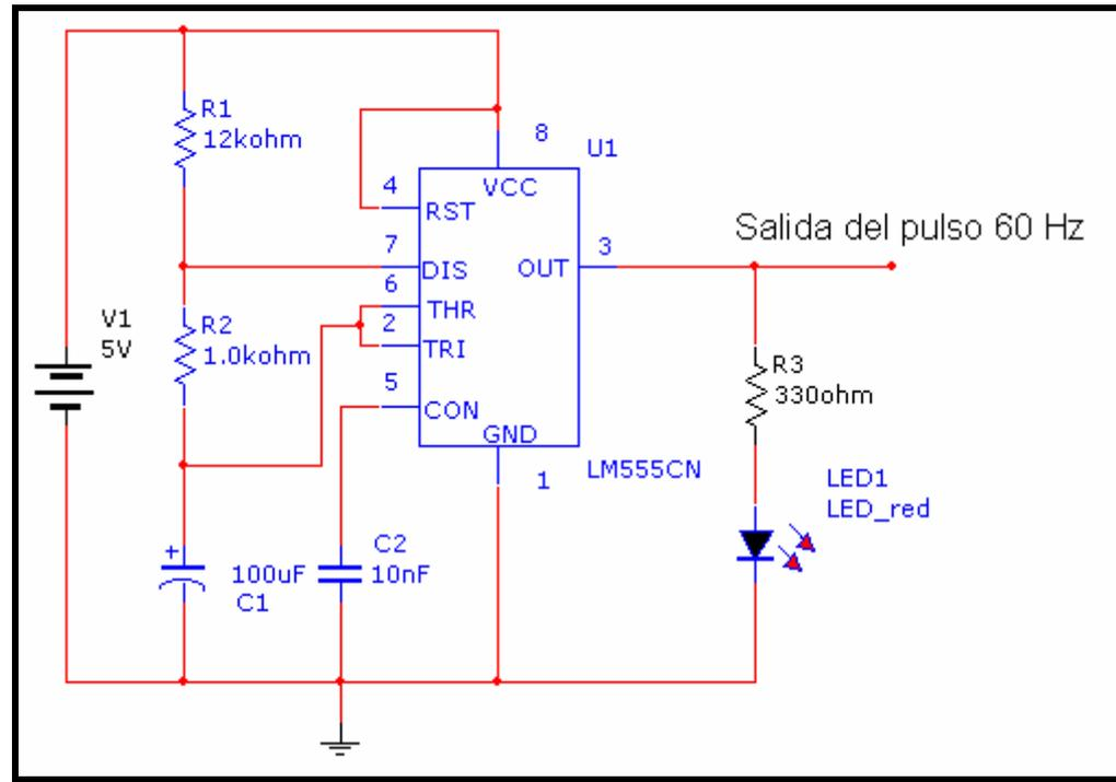
$$f = \frac{1.44}{(R1 + 2R2)C1} = \frac{1.44}{(12k\Omega + 2 * 1k\Omega)100\mu F} = 1.02857Hz$$
